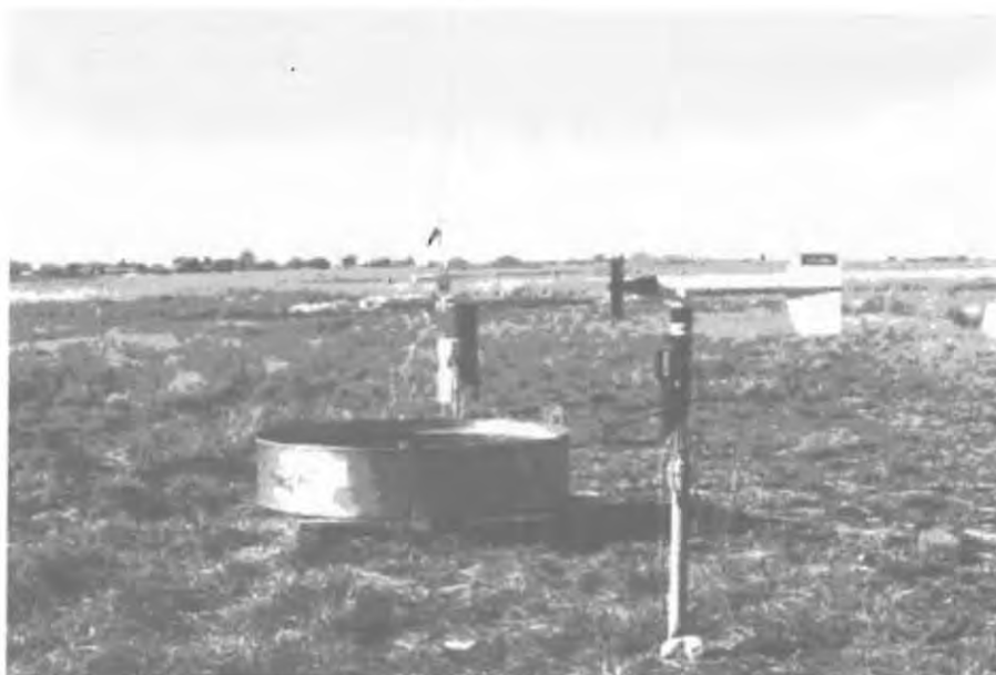
Figure 5: Class-A evaporation pan between the two lined dugouts at Swift Current; the 10-m meteorological tower is visible to the west of the pan (photo by G. Strong).
