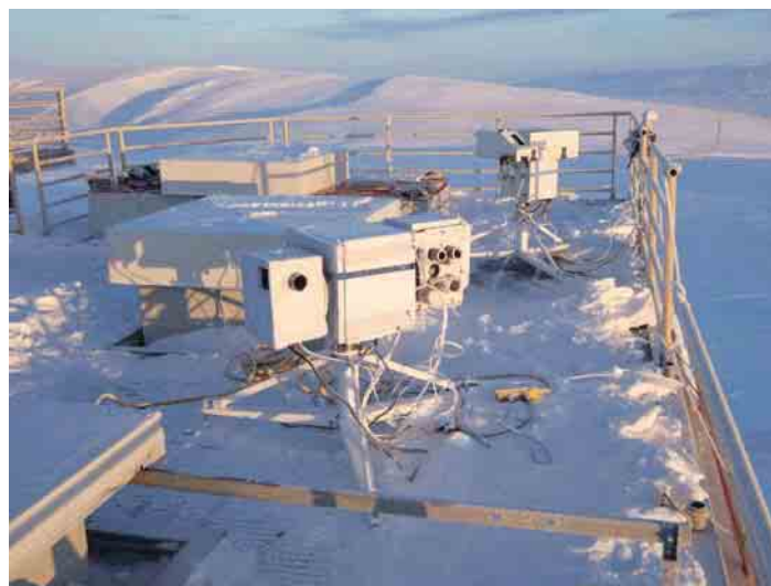
Figure 5: UV-visible instruments (SPS, MAESTRO-G and Brewer spectrophotometer) measuring atmospheric spectra from the rooftop at PEARL. (Photo by Tobias Kerzenmacher, March 2006)
