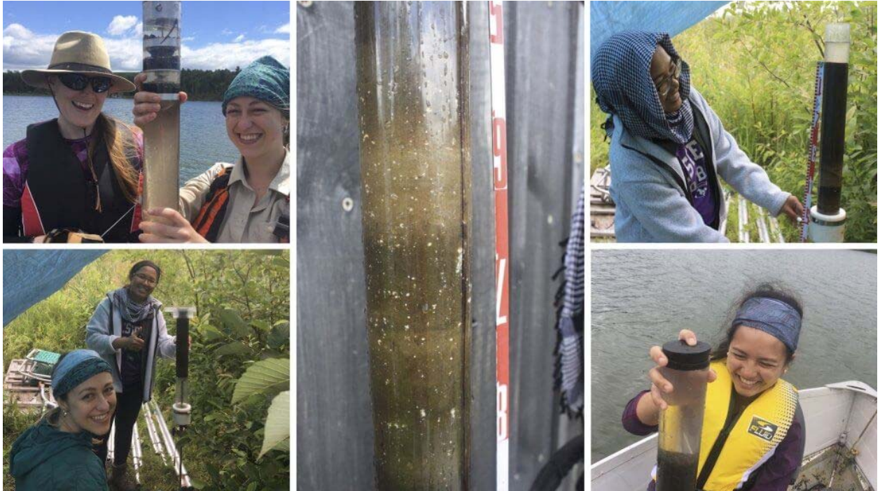
Figure 3. Sediment coring at Barry Lake, southeastern Ontario. Clockwise from top left: Carolyn Hill- Svehla and Rebecca Doyle with piston core top; sediment gravity core; Amanda Philavong with core extruder; Maria Sia with gravity core showing sediment-water interface; Rebecca Doyle and Amanda Philavong with sediment core extruder. Photographic credit: Western's Laboratory for Stable Isotope Science (LSIS) / Lake and Reservoir system Facility (LARS) coring team.
