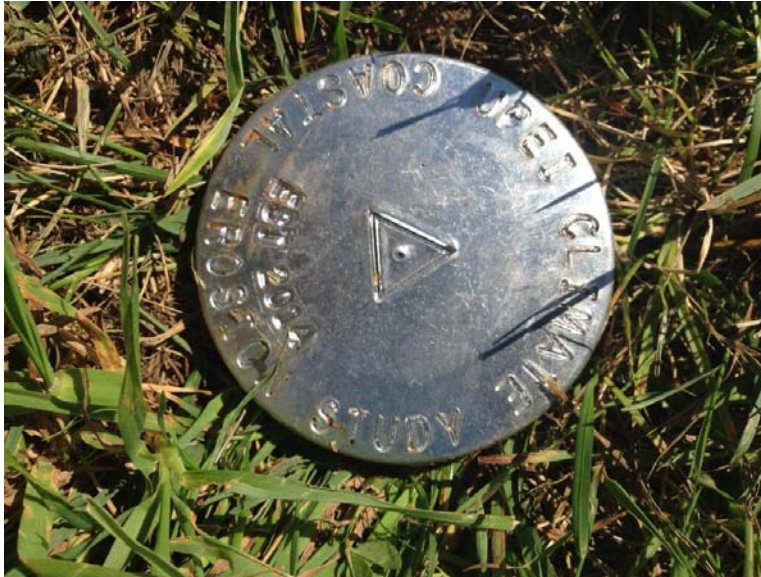
Figure 1: UPEI Climate Lab cap on peg for measuring coastal erosion year-to-year.
