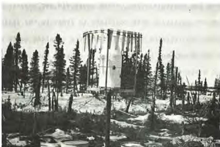
Fig. 5. The Fischer-Porter totalizing precipitation gauge installed near the McGill Laboratory.
