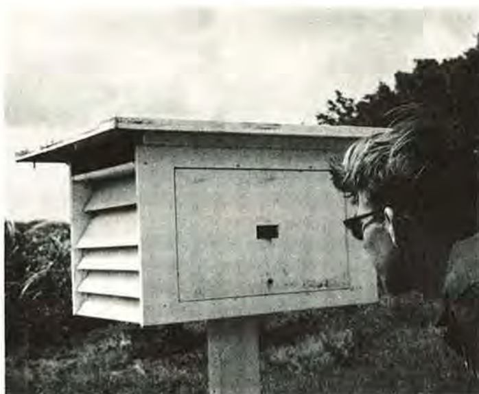
Fig. 4. Housing for Silicon Cell and Meter.
