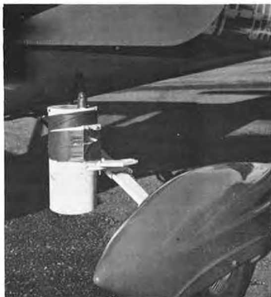
(a) PRT-5 installed on aircraft step.
