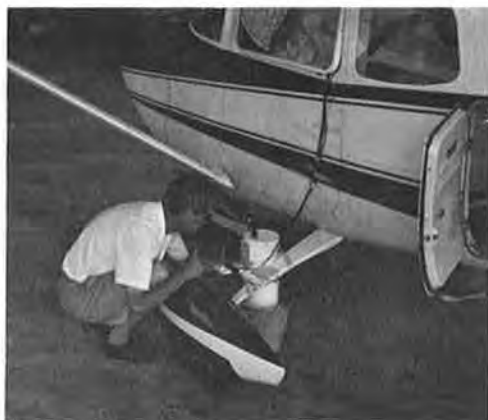
(a) PRT-5 installed on aircraft step.
