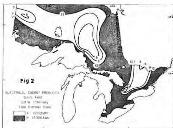
FIG 1 and FIG 2 SHOW THE ESTIMATED AMOUNT OF ELECTRICAL ENERGY per annum produced by 50% efficient (1) medium sized, and (2) large sized wind generators respectively. Energy loss in storage is not included.
