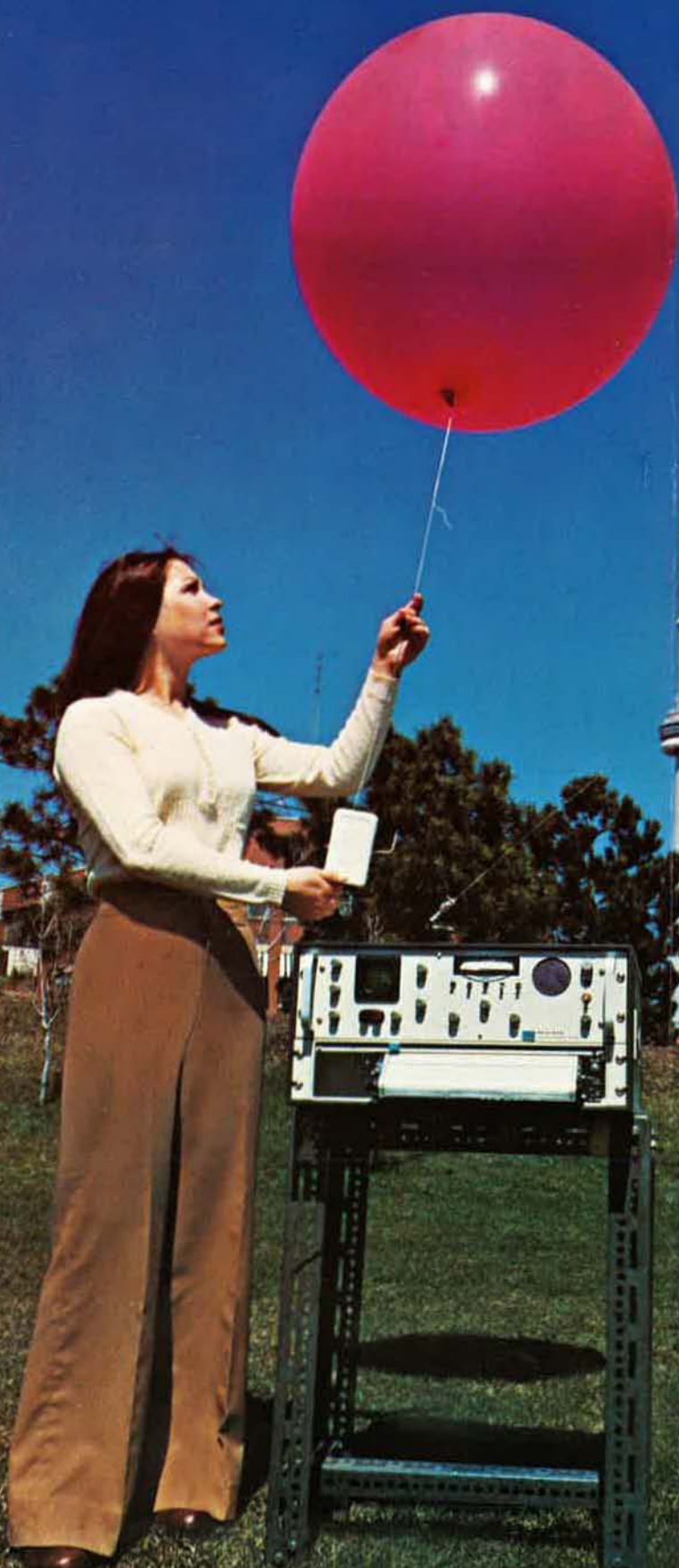
Launching Mini-T-Sonde, for Temperature and Wind Observations in Lower Atmosphere.
