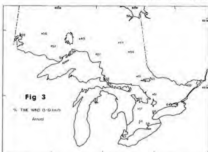
FIG 3 GIVES THE PERCENTAGE OF TIME during an average year that hourly wind speed readings fall between 13 and 61 km/h. This corresponds to the range of wind speeds in which most aerogenerators produce power.
