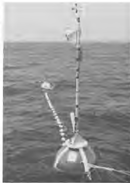
NOAA data buoy anchored offshore past the farthest yachting course. Data are automatically radioed to shore.
