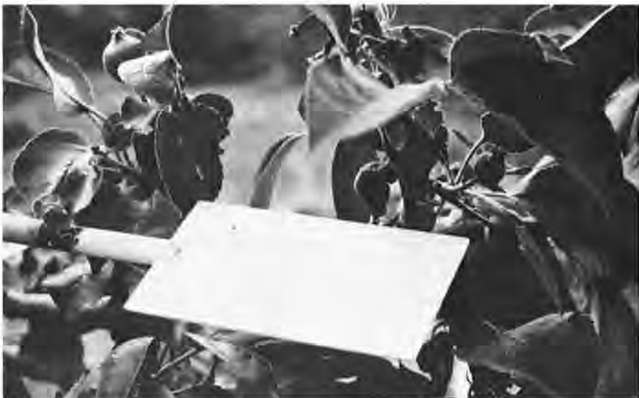
Flat plate used to measure duration of wetness on apple leaves.
