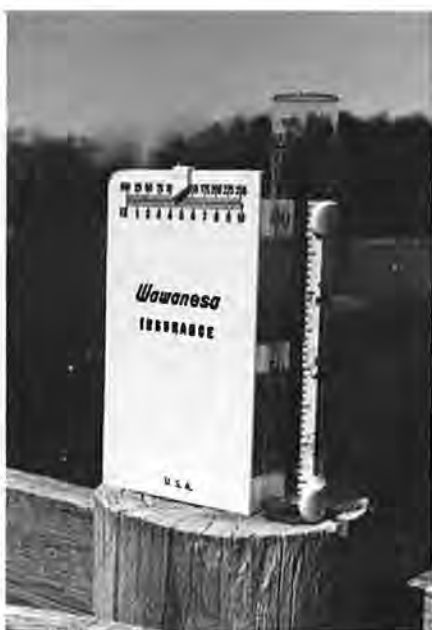
Figure 5 Different type of test-tube gauge made available to farmers by farm-support agencies in Saskatchewan.
