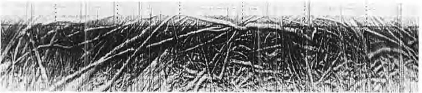
Figure 11 Sonograph showing a complex criss-crossing pattern of iceberg plough marks in about 380-m water depth on the uppermost continental slope west of Norway. Sonograph obtained using the IOS 31/37 kHz hull-mounted side-scan sonar system. Length of sonograph is 16.5 km, width 1.2 km (Courtesy: Institute of Oceanographic Sciences, Wormley, Surrey, United Kingdom).
