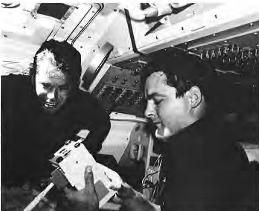
Marc Garneau conducting an experiment, as fellow astronaut Dave Leesma watches, on shuttle mission 41G using a "sunphotometer" designed by Environment Canada scientists.
