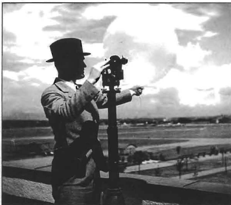
Pat Ryan, an aviation weather observer at Vancouver's Sea Island airport prepares to take a pilot balloon observation, circa 1936.
