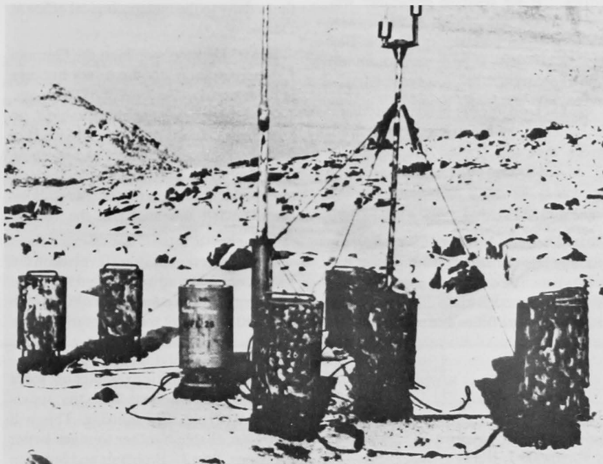
German automatic weather station WFL 26 as installed in Labrador, October 23, 1943. (Photo: courtesy Franz Selinger).
