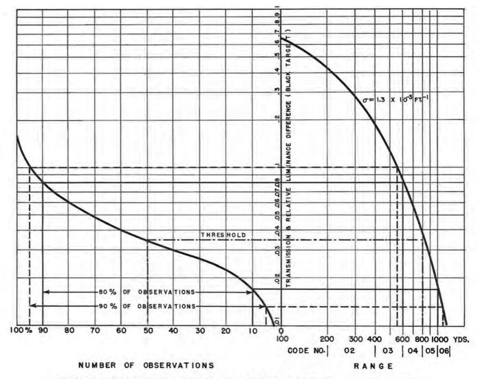
CURVES SHOWING PRECISION OF DETERMINATION OF VISUAL RANGE BY OBSERVATION OF CONVENTIONAL MARKS
