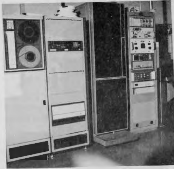
Control panel for VHRR in the SDL: showing interdata 7/16, M96 tape recorder and oscilloscope, receiver, antenna controller, discriminator, scan converter and synch detector from top to bottom in the right hand rack.
