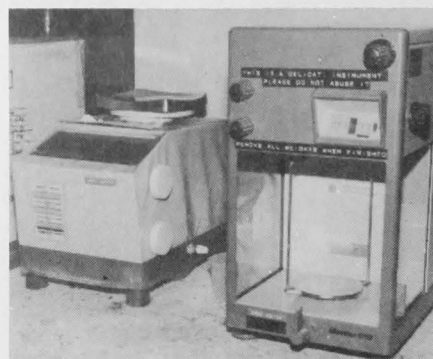
These are standard laboratory balances. The one on the right measures to the nearest ten thousandth of a gram; the one on the left to one tenth of a gram.
