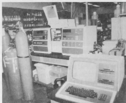
Less frequently used is the Atomic Absorption spectrophotometer, designed for the measurement of trace metal concentrations in samples collected from the atmosphere. The cylinders supply the fuel for the flame that is used in the analyses of samples.
