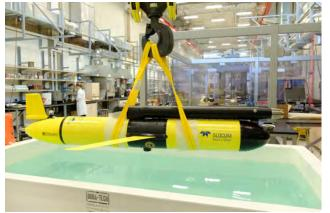
Figure 1: The UBC turbulent microstructureequipped ocean glider. The microstructure probes are mounted above and to the front of the instrument, at the end of the black cylindrical housing. Photo credit: Tara Howatt.
